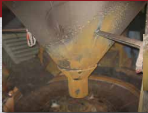
Structural and support members in the wear stream will benefit from GET Tungsten Carbide protection.
