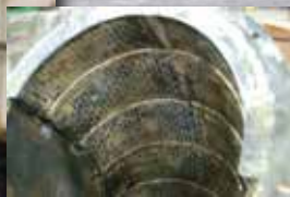
GET can apply Tungsten Carbide to all types of complex surfaces and shapes, such as this 45 degree elbow.
