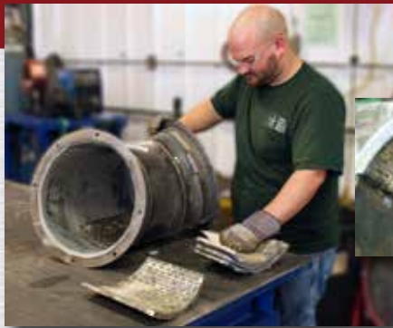
GET can apply Tungsten Carbide to all types of complex surfaces and shapes, such as this 45 degree elbow.
