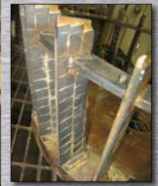
Good Earth Tools Carbide-protected classifier cages reduce downtime, typically lasting six times longer than the OEM.
