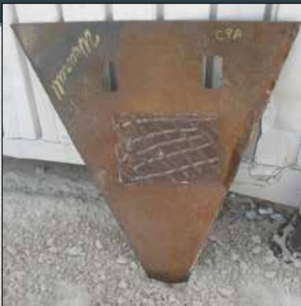
OEM headbox liners see a constant barrage of sand, wearing out quickly.
