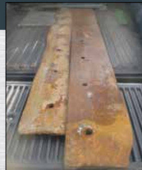
Worn steel hopper liners typically need replacing every six-eight months.
