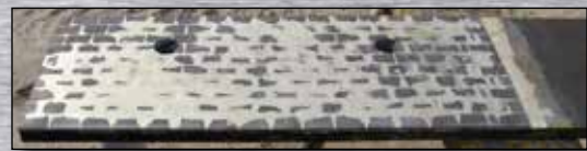
Good Earth Tools applies Carbide to the most critical area of the part.
