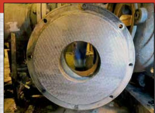
GET suction pump plate liners increase the life of the pump plate from four months to more than three years.
