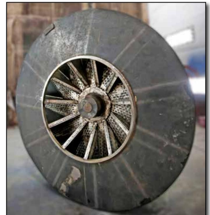
At 91 inches in diameter, this fan is a culmination of GET's detailed engineering, workmanship excellence, and more than 50 years of Carbide wear-proofing experience! GET produces the longest-lasting, most reliable fans on the market.
