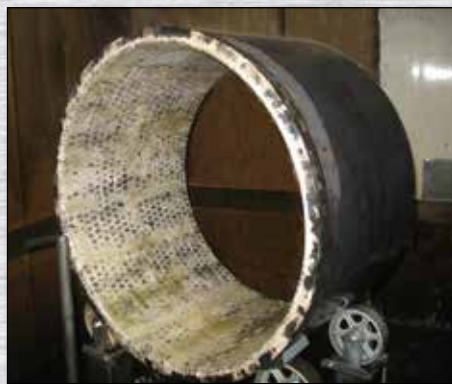
Good Earth Tools can apply solid Tungsten Carbide to a variety of surfaces, including this valve ring.
