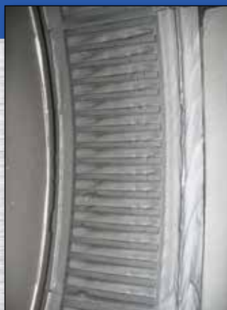
GET liner after 6,750 tons of processed limestone is ready for more jobs!
