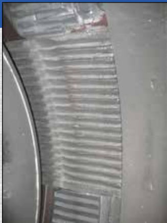
OEM casting after 1,500 tons of processed limestone is ready for "punch out".
