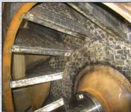
GET's custom Tungsten Carbide fan liner systems provide protection in critical wear areas.
