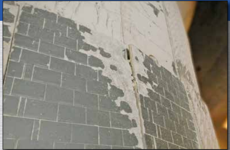
A GET solid Tungsten Carbide mill liner, still going strong after two years of service.
