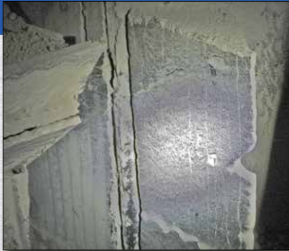
A competitor's chrome clad mill liner, in use for approximately six months and showing severe wear.
