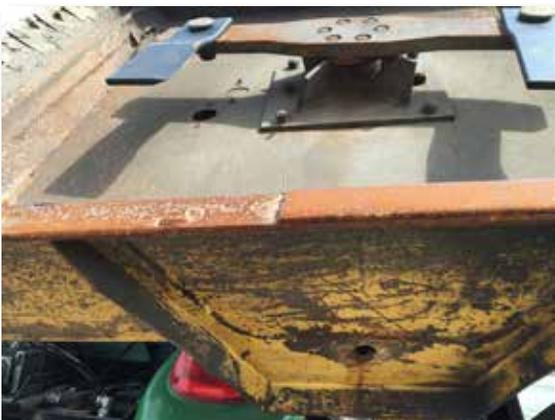
A skid on a mower without Z-Skid Carbide protection will quickly deteriorate and need replacing.
