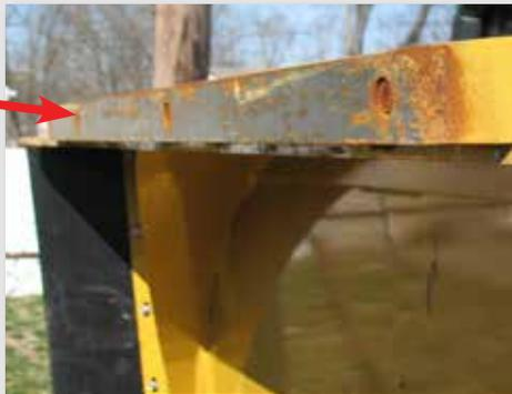
The OEM skid on a Tiger mower typically lasts just a few months, requiring a replacement about twice per mowing season.
